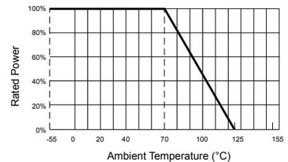
Maximum dissipation in percentage of rated power as a function of the ambient temperature for 0201, 01005
