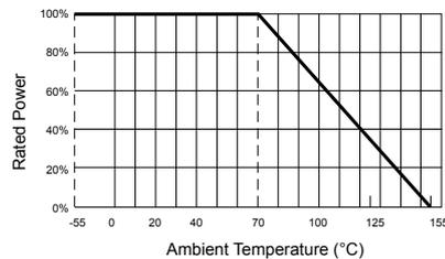
Maximum dissipation in percentage of rated power as a function of the ambient temperature for 0402, 0603, 0805, 1206, 1210, 2010, 2512
