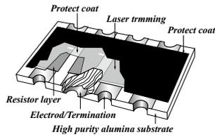
Fig 2. Construction of a Chip-R array (concave type)
