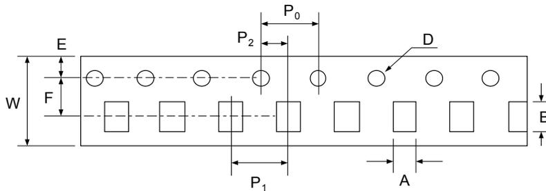
• Accumulated dimensional tolerance 40±0.2mm
