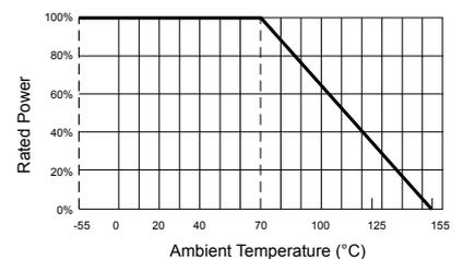
Maximum dissipation in percentage of rated power as a function of the ambient temperature for 0603, 0805, 1206, 1210, 2010, 2512
