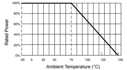
Maximum dissipation in percentage of rated power as a function of the ambient temperature for 0402, 0603, 0805, 1206, 1210, 2010, 2512, 1218
