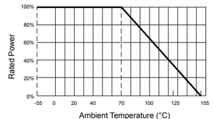
Maximum dissipation in percentage of rated power as a function of the ambient temperature
