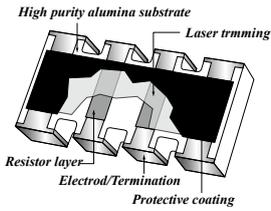
Fig 1. Construction of a Chip-R array (convex type)
